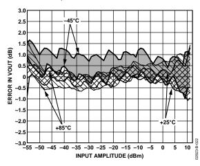
Figure 22. Logarithmic Law Conformance vs. Input Amplitude, 3 Sigma to Either Side of Mean, Sine Wave, Frequency 1900 MHz, Temperature –40°C, +25°C, and +85°C
