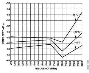
Figure 25. Logarithmic Intercept vs. Frequency, Temperature −40°C, +25°C, and +85°C
