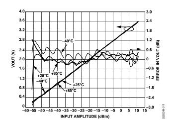
Figure 11. VOUT and Law Conformance vs. Input Amplitude, Frequency 1900 MHz, Sine Wave, Temperature −40°C, +25°C, and +85°C
