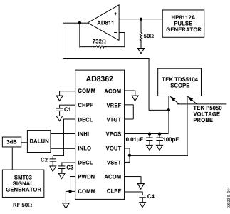
Figure 41. Response Measurement Setup for Gated Supply
