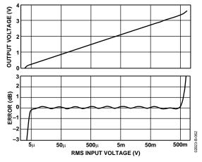
Figure 62. Output and Conformance for the AD8330/AD8362 Collaboration
