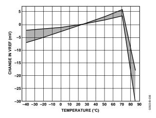
Figure 36. Change in VREF vs. Temperature, 3 Sigma to Either Side of Mean
