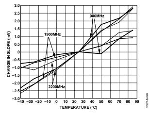
Figure 26. Change in Logarithmic Slope vs. Temperature, 3 Sigma to Either Side of Mean, Frequencies 900 MHz, 1900 MHz, 2200 MHz
