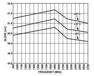
Figure 24. Logarithmic Slope vs. Frequency, Temperature −40°C, +25°C, and +85°C
