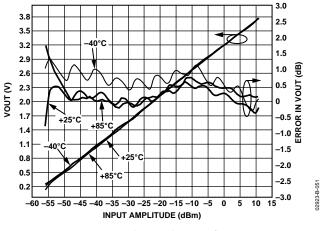
Figure 51. Output Voltage and Law Conformance Error, at  $T_A = -40^{\circ}$ C, +25°C, and +85°C
