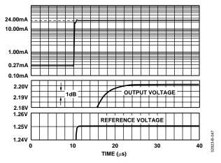
Figure 47. Typical Wake-Up Response;  $t_0 = 10 \, \mu s$
