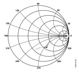
Figure 35. Input Impedance,  $Z_0 = 50 \Omega$ , Differential Drive
