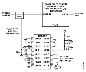
Figure 60. Generalized Control Loop Using the AD8362
