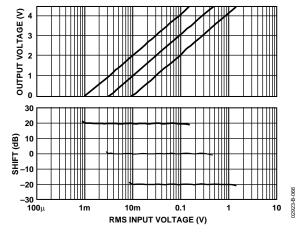
Figure 66. Illustrative Results for Slope of 100 mV/dB
