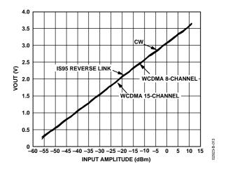
Figure 13. VOUT vs. Input Amplitude with Different Waveforms, CW, IS95 Reverse Link, WCDMA 8-Channel, WCDM 15-Channel, Frequency 900 MHz
