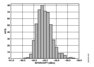
Figure 29. Logarithmic Intercept Distribution, Frequency 900 MHz
