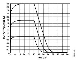
Figure 44. Typical Large-Scale Response
