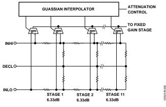
Figure 52. Simplified Input Circuit
