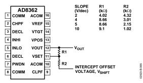
Figure 65. Slope and Intercept Adjustment
