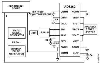
Figure 40. Response Measurement Setup for Power-Down Step
