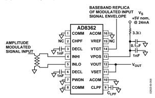
Figure 58. Envelope Elimination Using the VTGT Interface
