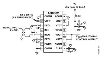
Figure 50. Connections for RF Power Measurement
