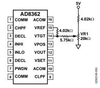
Figure 55. Adjustments of the Intercept by  $\pm 3 \, dB$
