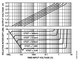
Figure 45. Response with VTGT Varied from 0.3 V to 3 V in 5 dB Steps, Showing the Proportional Shift in Intercept
