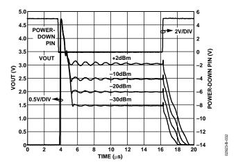
Figure 32. Output Response Using Power-Down Mode for Various RF Input Levels, Carrier Frequency 900 MHz, CLPF = 0
