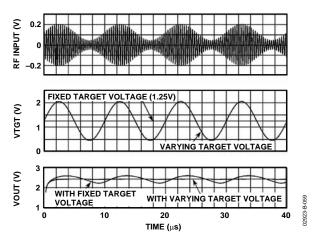
Figure 59. Waveforms for Envelope Elimination Scheme
