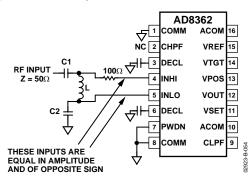
Figure 54. Narrow-Band Reactive Input Coupling
