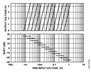
Figure 68. Illustrative Results for Slope of 10 mV/dec
