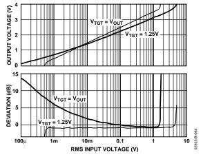
Figure 64. Dynamic Range Expansion Using VTGT = VOUT
