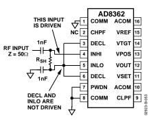
Figure 53. Input Coupling from a Single-Ended Source
