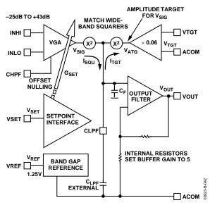
Figure 42. Basic Structure of the AD8362
