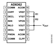
Figure 63. RF Power Meter with 80 dB Range
