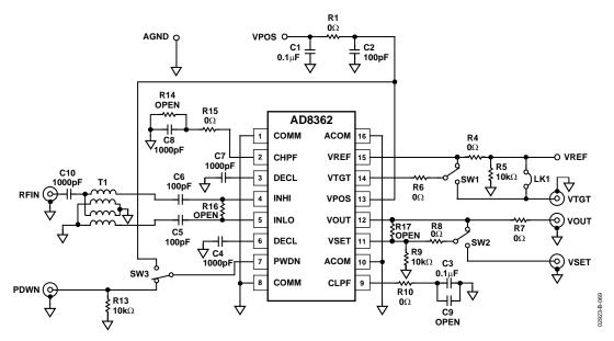
Figure 69. Evaluation Board Schematic
