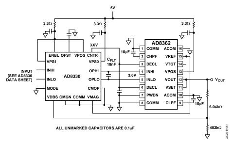
Figure 61. RMS Voltmeter with >100 dB Dynamic Range
