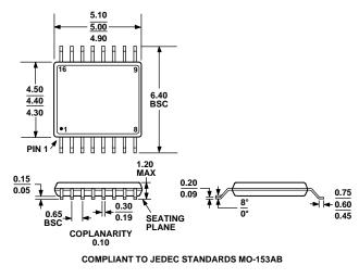
Figure 72. 16-Lead Thin Shrink Small Outline Package [TSSOP] (RU-16) Dimensions shown in millimeters
