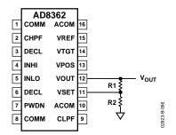
Figure 56. External Network to Raise Slope
