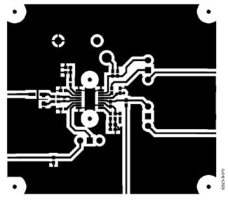
Figure 70. Component Side Metal of Evaluation Board
