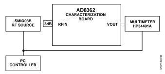
Figure 38. Primary Characterization Setup
