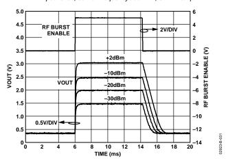
Figure 31. Output Response to RF Burst Input for Various RF Input Levels, Carrier Frequency 900 MHz, CLPF = 0.1 µF
