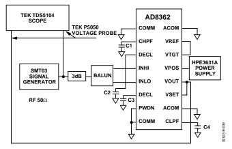
Figure 39. Response Measurement Setup for Modulated Pulse
