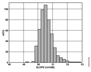
Figure 28. Slope Distribution, Frequency 900 MHz
