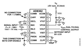
Figure 49. Basic Controller Mode Connections
