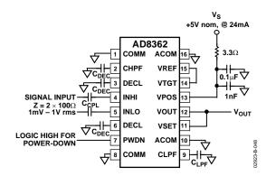
Figure 48. Basic Measurement Mode Connections
