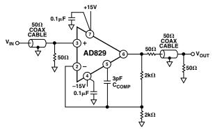
Figure 36. Noninverting Amplifier Connection Using Current Feedback Compensation
