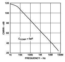
Figure 13. Common-Mode Rejection Ratio vs. Frequency
