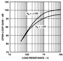
Figure 11. Open-Loop Gain vs. Resistive Load
