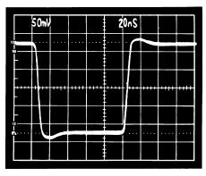
Figure 23c. Gain-of-20 Follower Small Signal Pulse Response
