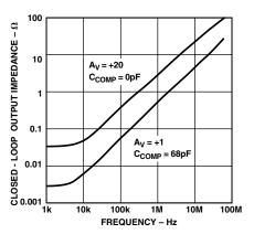
Figure 6. Closed-Loop Output Impedance vs. Frequency
