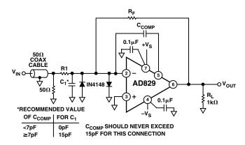
Figure 29. Inverting Amplifier Connection Using Current Feedback Compensation
