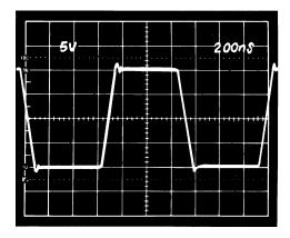
Figure 32. Large Signal Pulse Response of the Inverting Amplifier Using Current Feedback Compensation.  $C_{COMP} = 1$  pF,  $R_F = 3$  k $\Omega$ , R1 = 3 k $\Omega$
