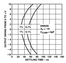
Figure 15. Output Swing & Error vs. Settling Time
