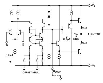
Figure 25. AD829 Simplified Schematic
