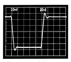
Figure 24c. Unity Gain Inverter Small Signal Pulse Response
