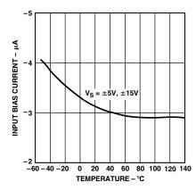
Figure 5. Input Bias Current vs. Temperature
