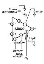
Figure 21. Offset Null and External Shunt Compensation Connections
