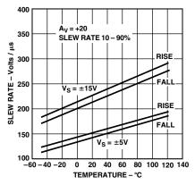
Figure 19. Slew Rate vs. Temperature
