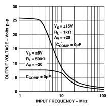
Figure 14. Large Signal Frequency Response
