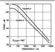
Figure 12. Power Supply Rejection Ratio (PSRR) vs. Frequency
