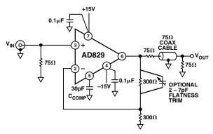
Figure 37. A Video Line Driver with a Flatness over Frequency Adjustment
