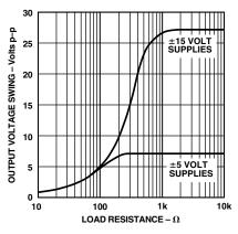
Figure 3. Output Voltage Swing vs. Resistive Load
