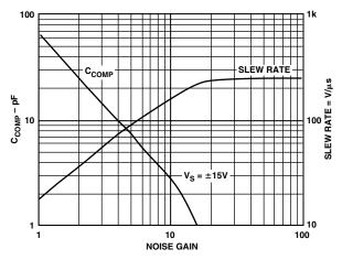
Figure 28. Value of C<sub>COMP</sub> & Slew Rate vs. Noise Gain
