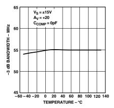
Figure 9. –3 dB Bandwidth vs. Temperature
