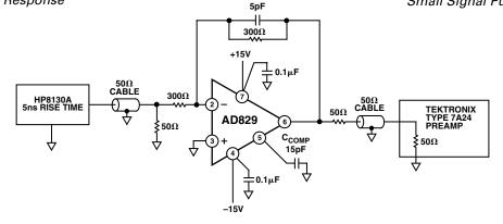
Figure 24a. Unity Gain Inverter Connection
