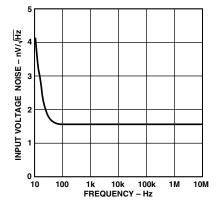
Figure 18. Input Voltage Noise Spectral Density
