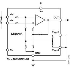
Figure 14. Ground Referenced Output
