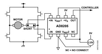
Figure 21. Motor Control Application
