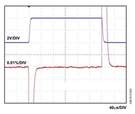
Figure 11. Settling Time
