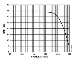
Figure 7. Typical Small Signal Bandwidth (Vout = 200 mV p-p)
