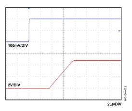
Figure 10. Differential Overload Recovery (Rising)
