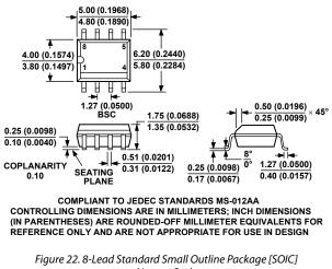
Narrow Body (R-8) Dimensions shown in millimeters and (inches)
