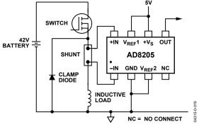
Figure 20. High-Side Switch
