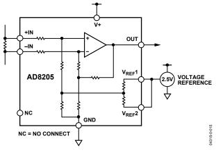
Figure 16. External Reference Output
