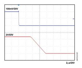
Figure 9. Differential Overload Recovery (Falling)
