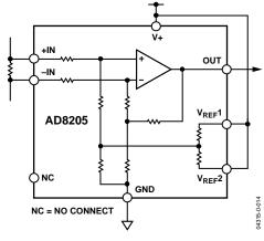
Figure 15. V+ Referenced Output
