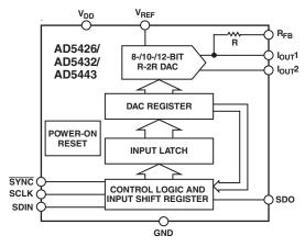
4-Quadrant Multiplication Power-On Reset with Brownout Detection Daisy-chain Mode Readback Function 0.4 μA Typical Power Consumption APPLICATIONS Portable Battery-Powered Applications Waveform Generators Analog Processing Instrumentation Applications
