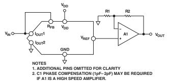
Figure 9. Single-Supply Voltage Switching Mode Operation
