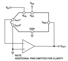
Figure 12. Current Steering DAC Used as a Divider or Programmable Gain Element
