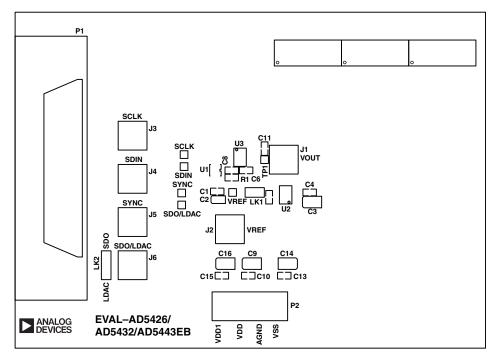
Figure 20. Silkscreen—Component Side View (Top Layer)
