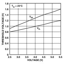
TPC 28. Threshold Voltages vs. Supply Voltage
