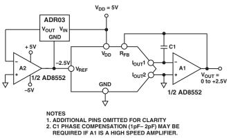
Figure 10. Positive Voltage Output with Minimum of Components
