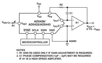
Figure 6. Unipolar Operation
