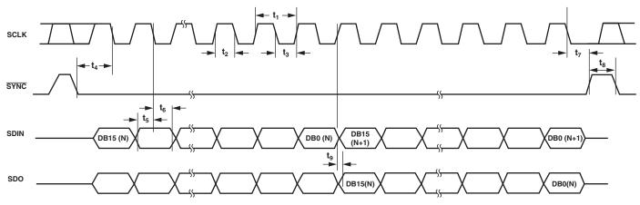
ALTERNATIVELY, DATA MAY BE CLOCKED INTO INPUT SHIFT REGISTER ON RISING EDGE OF SCLK AS DETERMINED BY CONTROL BITS. IN THIS CASE, DATA WOULD BE CLOCKED OUT OF SDO ON FALLING EDGE OF SCLK. TIMING AS PER ABOVE, WITH SCLK INVERTED.
