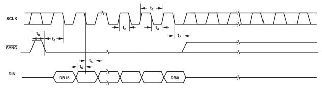
ALTERNATIVELY, DATA MAY BE CLOCKED INTO INPUT SHIFT REGISTER ON RISING EDGE OF SCLK AS DETERMINED BY CONTROL BITS. TIMING AS PER ABOVE, WITH SCLK INVERTED.
