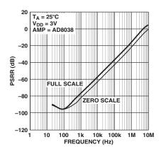
TPC 25. Power Supply Rejection vs. Frequency
