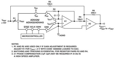
Figure 7. Bipolar Operation
