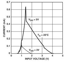
TPC 16. Supply Current vs. Logic Input Voltage,  $\overline{SYNC}$ (SCLK, DATA = 0)
