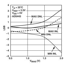
TPC 15. Linearity vs.  $V_{BIAS}$ Voltage Applied to  $I_{OUT2}$
