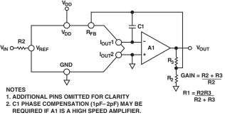
Figure 11. Increasing Gain of Current Output DAC
