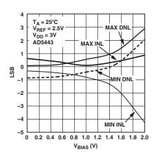
TPC 11. Linearity vs. V<sub>BIAS</sub> Voltage Applied to I<sub>OUT2</sub>
