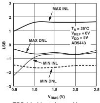
TPC 14. Linearity vs.  $V_{BIAS}$ Voltage Applied to  $I_{OUT2}$
