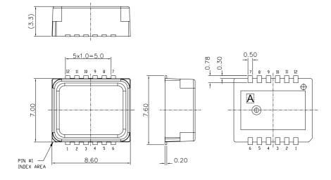
Figure 3. Housing dimensions
