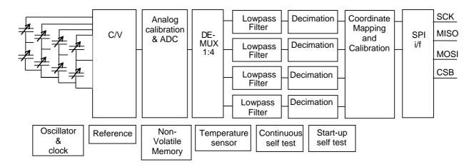
Figure 1. SCA3100-D07 Block diagram
