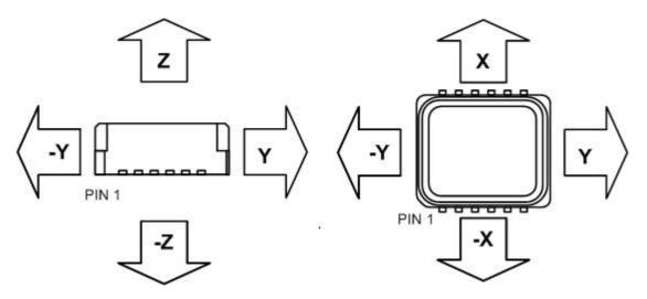
Figure 2. Accelerometer measuring directions
