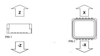
Figure 2. Accelerometer measuring directions
