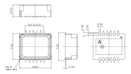
Figure 3. Housing dimensions
