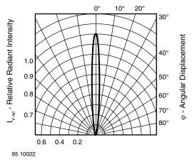
Figure 2. Relative Intensity vs. Angular Displacement
