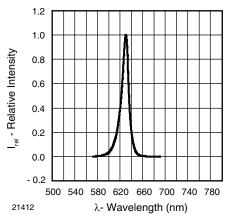
Figure 3. Relative Intensity vs. Wavelength
