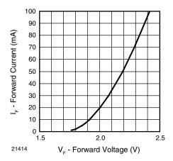
Figure 4. Forward Current vs. Forward Voltage
