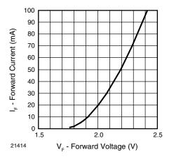
Figure 4. Forward Current vs. Forward Voltage
