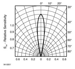
Figure 2. Relative Intensity vs. Angular Displacement
