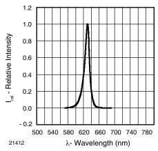
Figure 3. Relative Intensity vs. Wavelength
