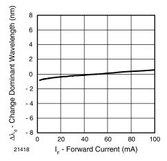
Figure 6. Change of Dominant Wavelength vs. Forward Current
