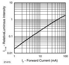
Figure 5. Relative Luminous Intensity vs. Forward Current
