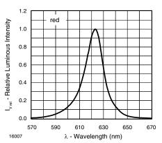
Figure 4. Relative Intensity vs. Wavelength
