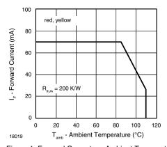
Figure 1. Forward Current vs. Ambient Temperature
