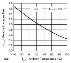
Figure 12. Rel. Luminous Flux vs. Ambient Temperature
