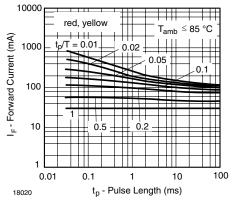
Figure 2. Forward Current vs. Pulse Length
