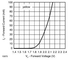
Figure 7. Forward Current vs. Forward Voltage
