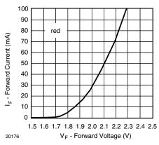
Figure 6. Forward Current vs. Forward Voltage
