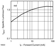
Figure 10. Specific Luminous Flux vs. Forward Current
