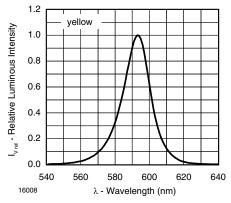
Figure 5. Relative Intensity vs. Wavelength
