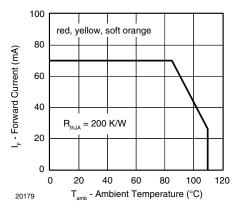
Figure 1. Forward Current vs. Ambient Temperature
