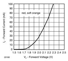
Figure 7. Forward Current vs. Forward Voltage
