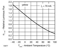
Figure 14. Rel. Luminous Flux vs. Ambient Temperature
