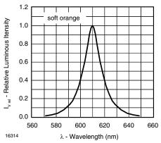
Figure 6. Relative Intensity vs. Wavelength
