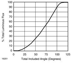
Figure 16. Percentage Total Luminous Flux vs. Total Included Angle for 90° Emission Angle
