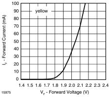
Figure 8. Forward Current vs. Forward Voltage
