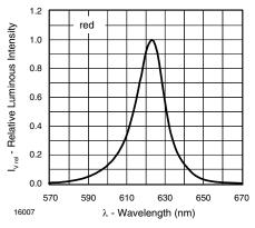
Figure 4. Relative Intensity vs. Wavelength
