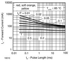
Figure 2. Forward Current vs. Pulse Length
