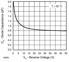
Figure 2. Diode Capacitance vs. Reverse Voltage
