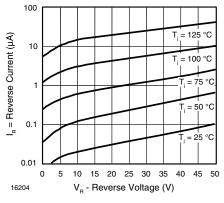
Figure 1. Reverse Current vs. Reverse Voltage
