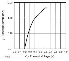
Figure 3. Forward Current vs. Forward Voltage
