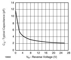
Figure 2. Typical Capacitance °C vs. Reverse Applied Voltage V<sub>R</sub>
