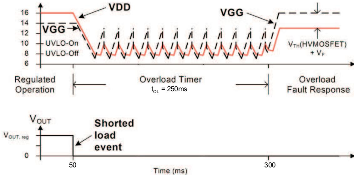
**Figure 32. Overload Behavior with a Shorted Output**
