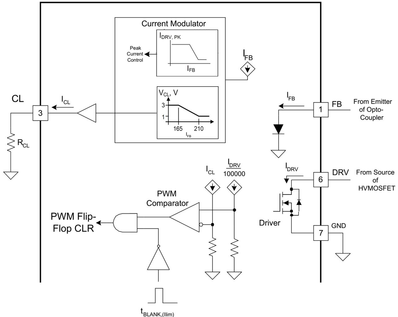
Figure 27. CL pin and DRV Current Sense
