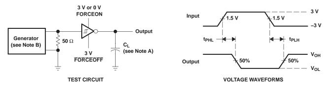
NOTES: A. C<sub>L</sub> includes probe and jig capacitance. B. The pulse generator has the following characteristics:  $Z_0 = 50 \ \Omega$ , 50% duty cycle,  $t_r \le 10 \text{ ns}$ ,  $t_f \le 10 \text{ ns}$ .
