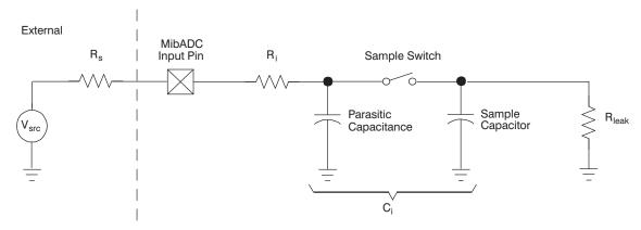
Figure 18. MibADC Input Equivalent Circuit
