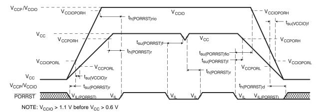
Figure 8. PORRST Timing Diagram
