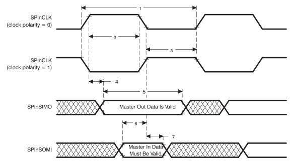
Figure 12. SPIn Master Mode External Timing (CLOCK PHASE = 0)
