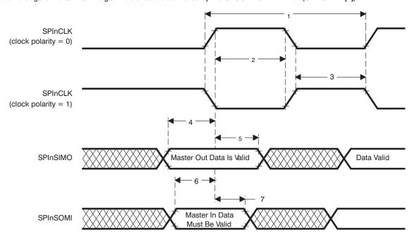
Figure 13. SPIn Master Mode External Timing (CLOCK PHASE = 1)
