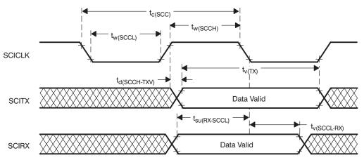
Data transmission / reception characteristics for isosynchronous mode with external clocking are similar to the asynchronous mode. Data transmission occurs on the SCICLK rising edge, and data reception occurs on the SCICLK falling edge.
