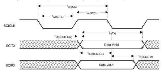
Data transmission/reception characteristics for isosynchronous mode with internal clocking are similar to the asynchronous mode. Data transmission occurs on the SCICLK rising edge, and data reception occurs on the SCICLK falling edge.
