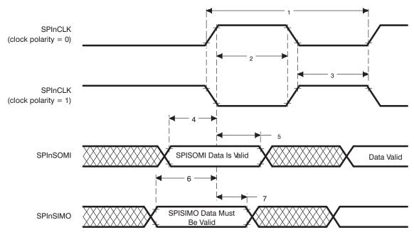
Figure 15. SPIn Slave Mode External Timing (CLOCK PHASE = 1)
