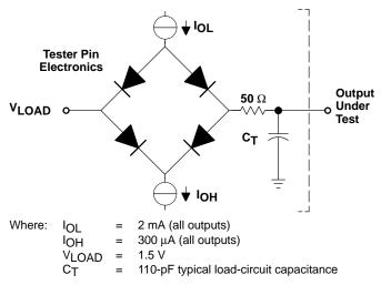
Figure 17. Test Load Circuit
