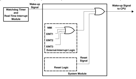
Figure 9. Waking Up the Device From Power Down
