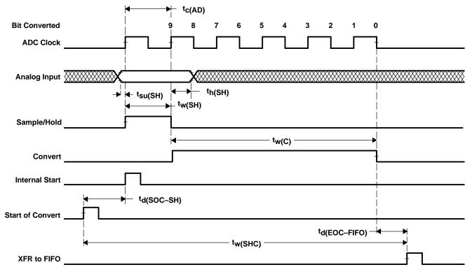
Figure 49. Analog-to-Digital Timing
