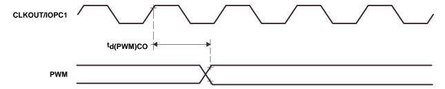
Figure 35. PWM and Compare Output Timings
