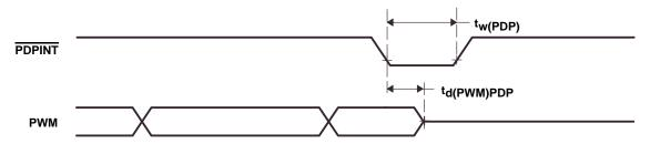
Figure 40. Power-Drive Protection Interrupt Timings
