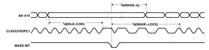
Figure 25. PLL Power-Down Entry and Exit Timings
