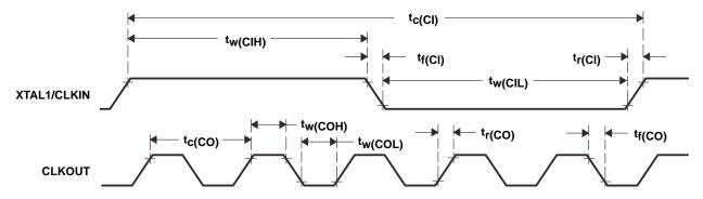
Figure 22. CLKIN-to-CLKOUT Timings for PLL Oscillator Mode, Multiply-by-5 Option With 4-MHz Crystal
