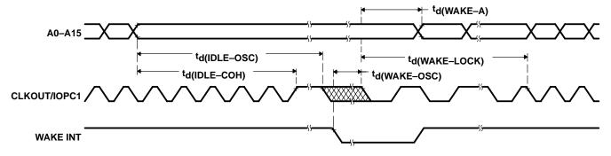
Figure 26. OSC Power-Down Entry and Exit Timings
