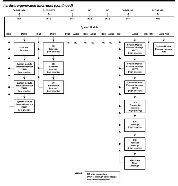
Figure 6. System Module Interrupt Structure
