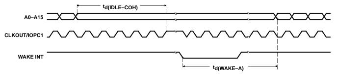
Figure 24. IDLE2 Entry and Exit Timings
