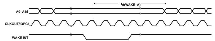
Figure 23. IDLE1 Entry and Exit Timings
