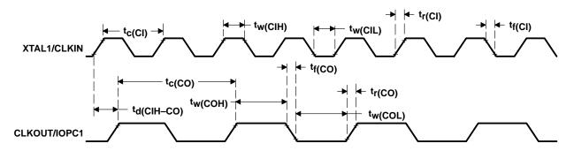
Figure 21. External Divide-by-Two Clock Timings
