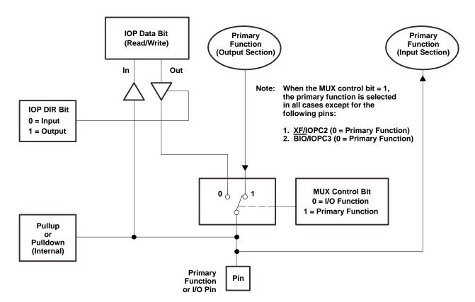
Figure 3. Shared Pin Configuration
