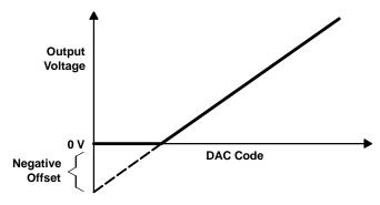
Figure 15. Effect of Negative Offset (Single Supply)
