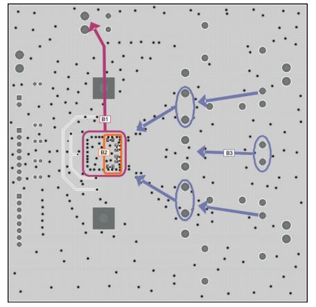
**Note B1**: It is important to have a direct low impedance return path for high current back to the power supply. Keep impedance low from top to bottom side of PCB through a lot of ground vias.
