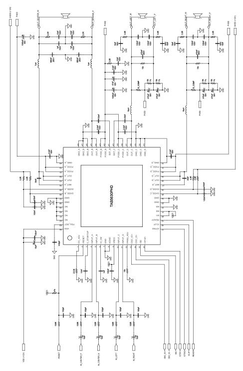
Figure 17. Typical 2.1 System Differential Input BTL and Unbalanced Input SE Application
