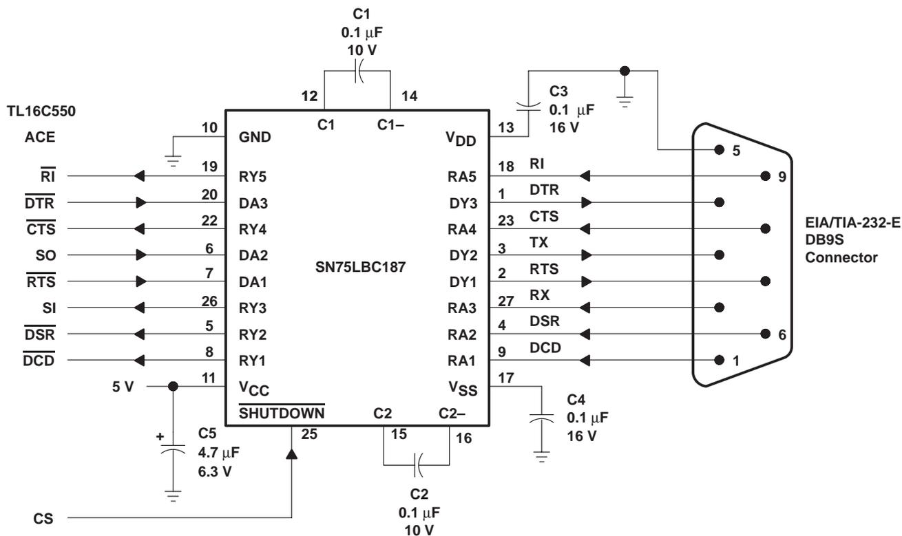
NOTE: C1, C2, C3, and C4 are Z5U-type ceramic-chip capacitors.
