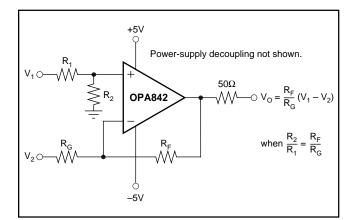
FIGURE 3. High-Speed, Single Differential Amplifier.
