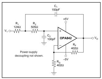
FIGURE 6. 5MHz Butterworth Low-Pass Active Filter.
