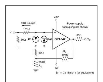
FIGURE 9. Gain of +2 with Input Protection.
