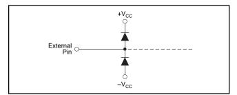
FIGURE 8. Internal ESD Protection.
