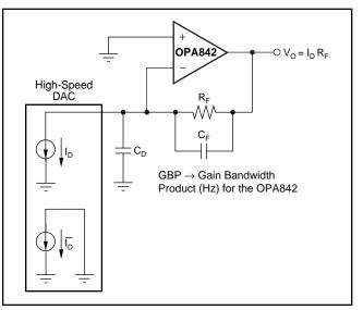
FIGURE 5. Wideband Low-Distortion DAC Transimpedance Amplifier.
