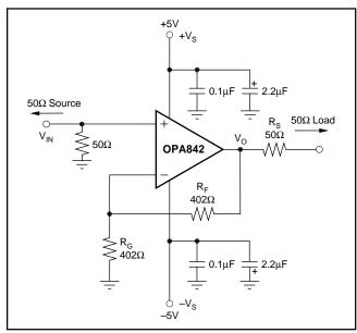
FIGURE 1. Gain of +2. High-frequency application and characterization circuit.
