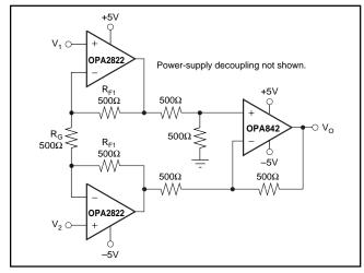
FIGURE 4. Wideband 3-Op Amp Differencing Amplifier.
