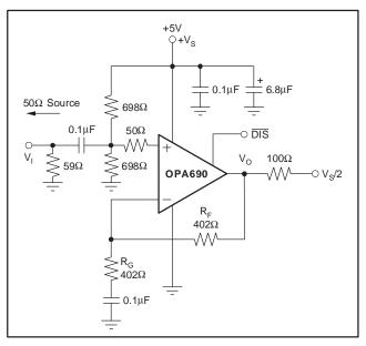
Figure 2. DC-Coupled, G = +2, Single-Supply, Specification and Test Circuit
