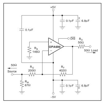
Figure 8. Gain of -2 Example Circuit
