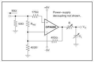
Figure 9. Capacitive Load Driving with Noise Gain Tuning
