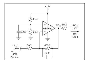
Figure 6. High-Power Coax Line Driver
