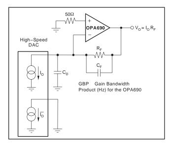
Figure 5. DAC Transimpedance Amplifier
