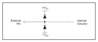
Figure 15. Internal ESD Protection
