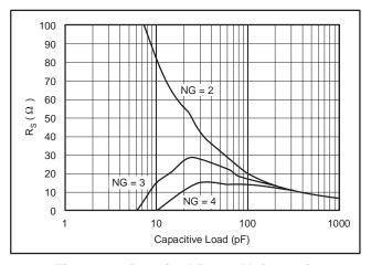
Figure 10. Required R<sub>S</sub> vs Noise Gain
