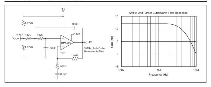
Figure 7. Single-Supply, High-Frequency Active Filter
