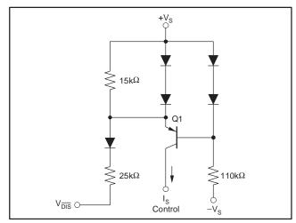
Figure 13. Simplified Disable Control Circuit
