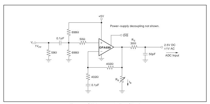
Figure 4. SFDR versus IB Test Circuit
