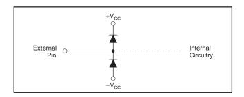
Figure 16. ESD Steering Diodes
