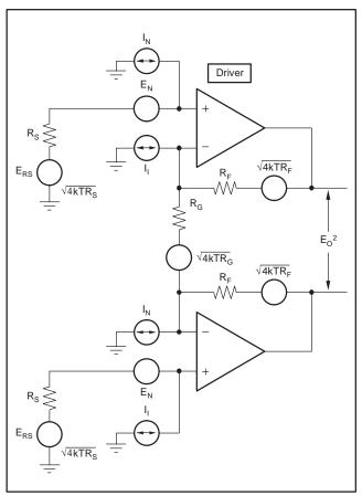
Figure 14. Differential Op Amp Noise Analysis Model
