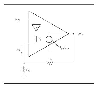
Figure 10. Current-Feedback Transfer Function
