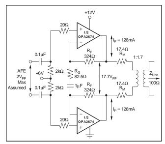
Figure 5. Single-Supply ADSL Upstream Driver
