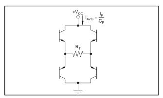
Figure 9. Output Stage Power Model
