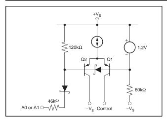
Figure 15. Supply Power Control Circuit
