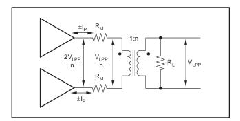
Figure 7. Driver Peak Output Model
