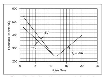
Figure 11. Feedback Resistor vs Noise Gain
