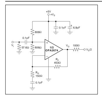
Figure 3. AC-Coupled, G = +4, Single-Supply, Specification and Test Circuit
