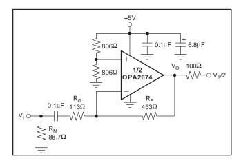
Figure 4. AC-Coupled, G = -4, Single-Supply, Specification and Test Circuit
