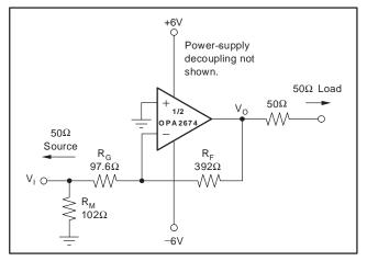
Figure 12. Inverting Gain of -4 with Impedance Matching
