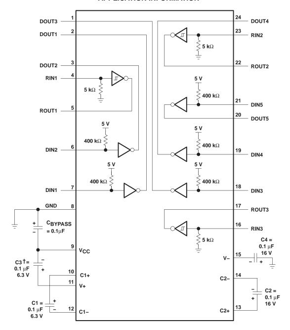
$^\dagger\text{C3}$  can be connected to  $\text{V}_{\mbox{CC}}$  or GND.
