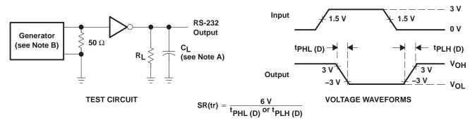
NOTES: A. CL includes probe and jig capacitance.
