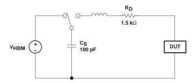
Figure 5. HBM ESD Test Circuit
