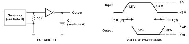
NOTES: A. C<sub>L</sub> includes probe and jig capacitance.
