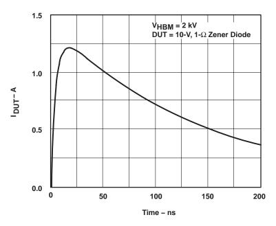
Figure 6. Typical HBM Current Waveform
