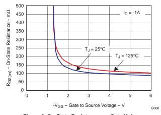
Figure 6. On-State Resistance vs. Gate Voltage
