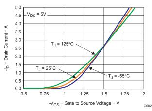
Figure 3. Transfer Characteristics
