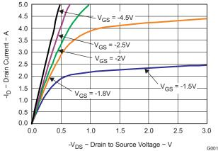
Figure 2. Saturation Characteristics
