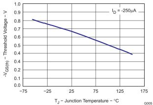
Figure 12. Threshold Voltage vs. Temperature
