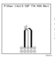
Max  $R_{\theta JA} = 212^{\circ} C/W$  when mounted on minimum pad area of 2-oz. (0.071-mm thick) Cu.
