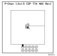
Max  $R_{\theta JA} = 119^{\circ}\text{C/W}$  when mounted on 1 inch<sup>2</sup> (6.45 cm<sup>2</sup>) of 2-oz. (0.071-mm thick) Cu.
