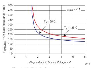
Figure 7. On-State Resistance vs. Gate Voltage
