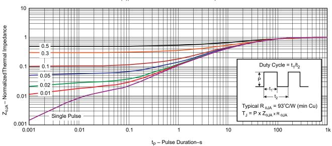
Figure 1. Transient Thermal Impedance
