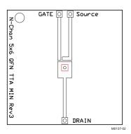
Max  $R_{\theta JA} = 115^{\circ}C/W$ when mounted on minimum pad area of 2-oz.Cu.
