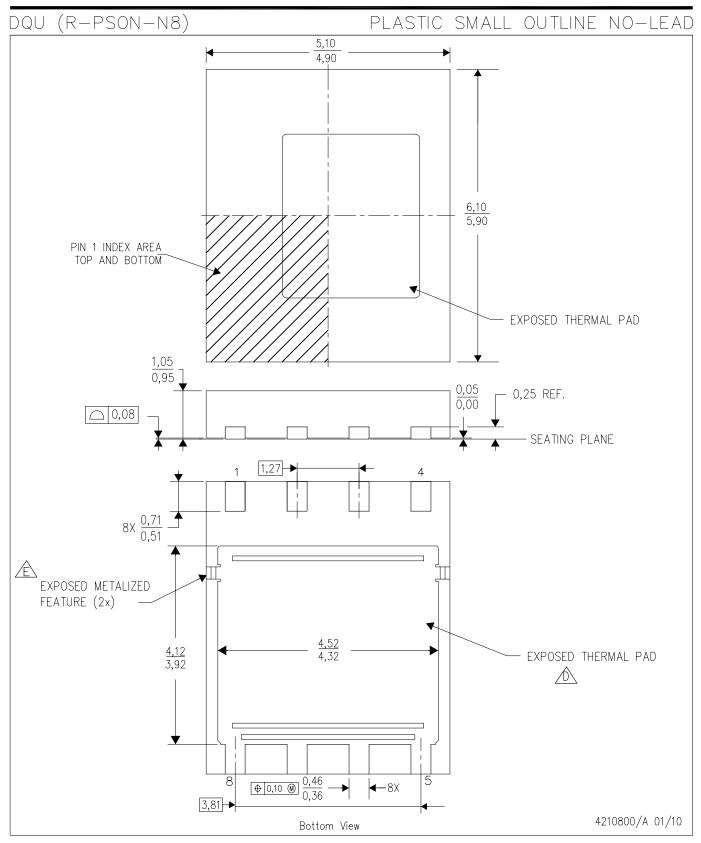
NOTES: A. All linear dimensions are in millimeters. Dimensioning and tolerancing per ASME Y14.5M-1994.
