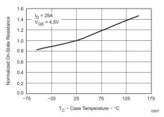
Figure 8. On Resistance vs. Temperature
