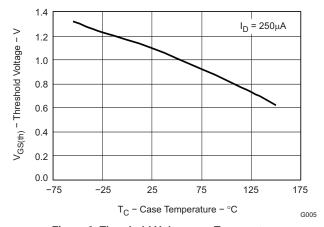
Figure 6. Threshold Voltage vs. Temperature
