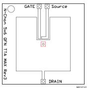
Max  $R_{\theta JA} = 48^{\circ}C/W$ when mounted on 1 in<sup>2</sup> of 2-oz. Cu.
