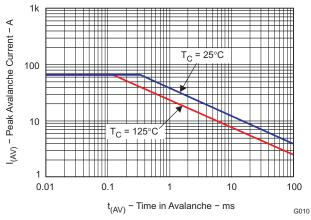
Figure 11. Single Pulse Unclamped Inductive Switching
