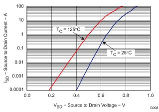
Figure 9. Typical Diode Forward Voltage
