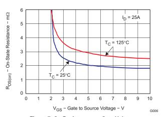
Figure 7. On Resistance vs. Gate Voltage
