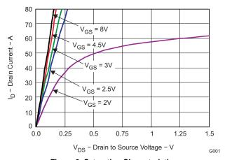
Figure 2. Saturation Characteristics
