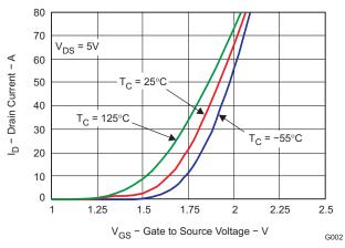
Figure 3. Transfer Characteristics
