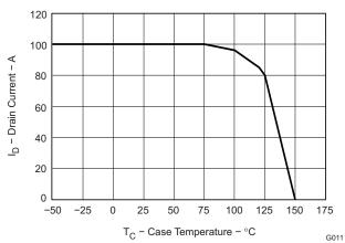
Figure 12. Maximum Drain Current vs. Temperature
