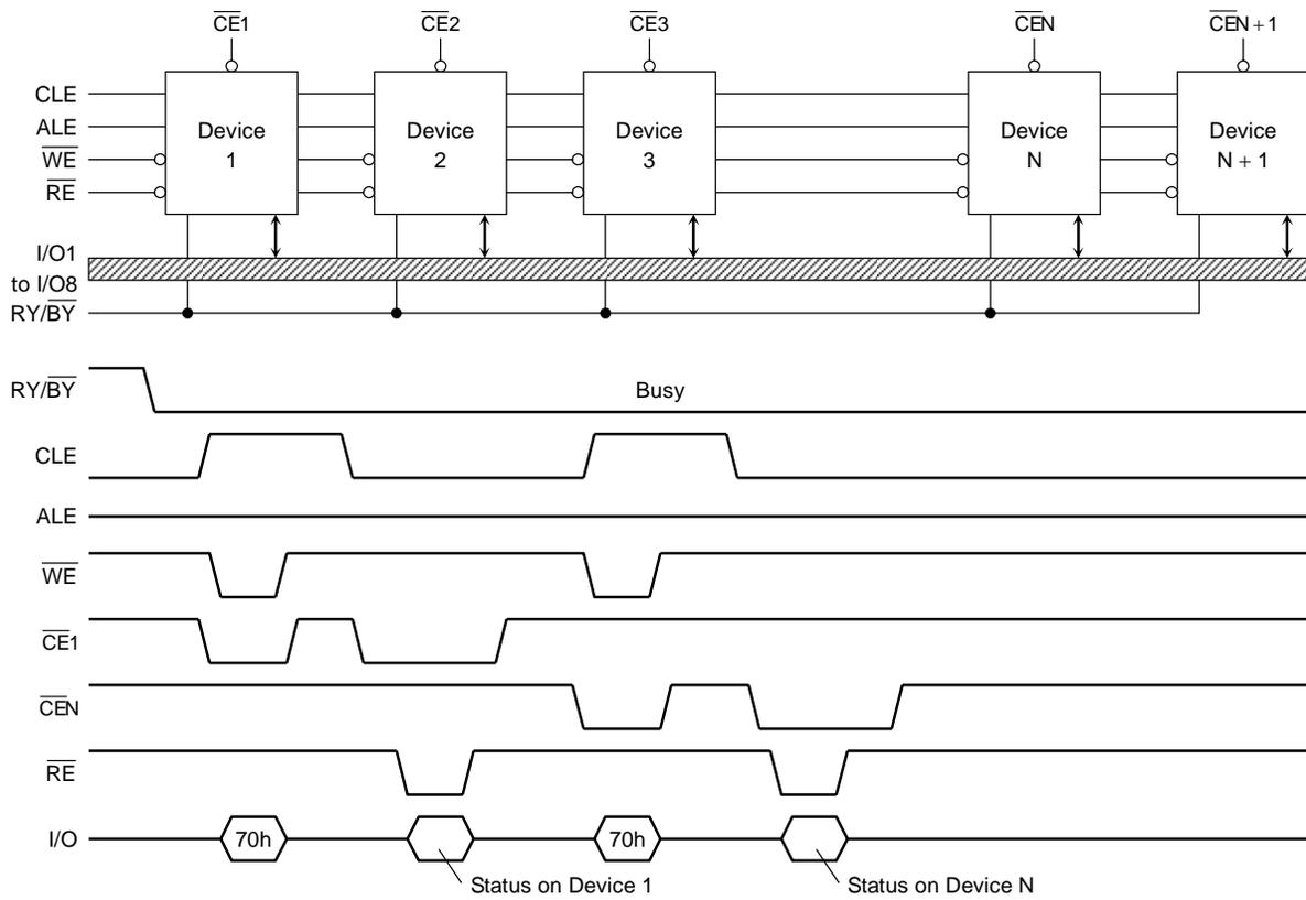
Figure 5. Status Read timing application example
