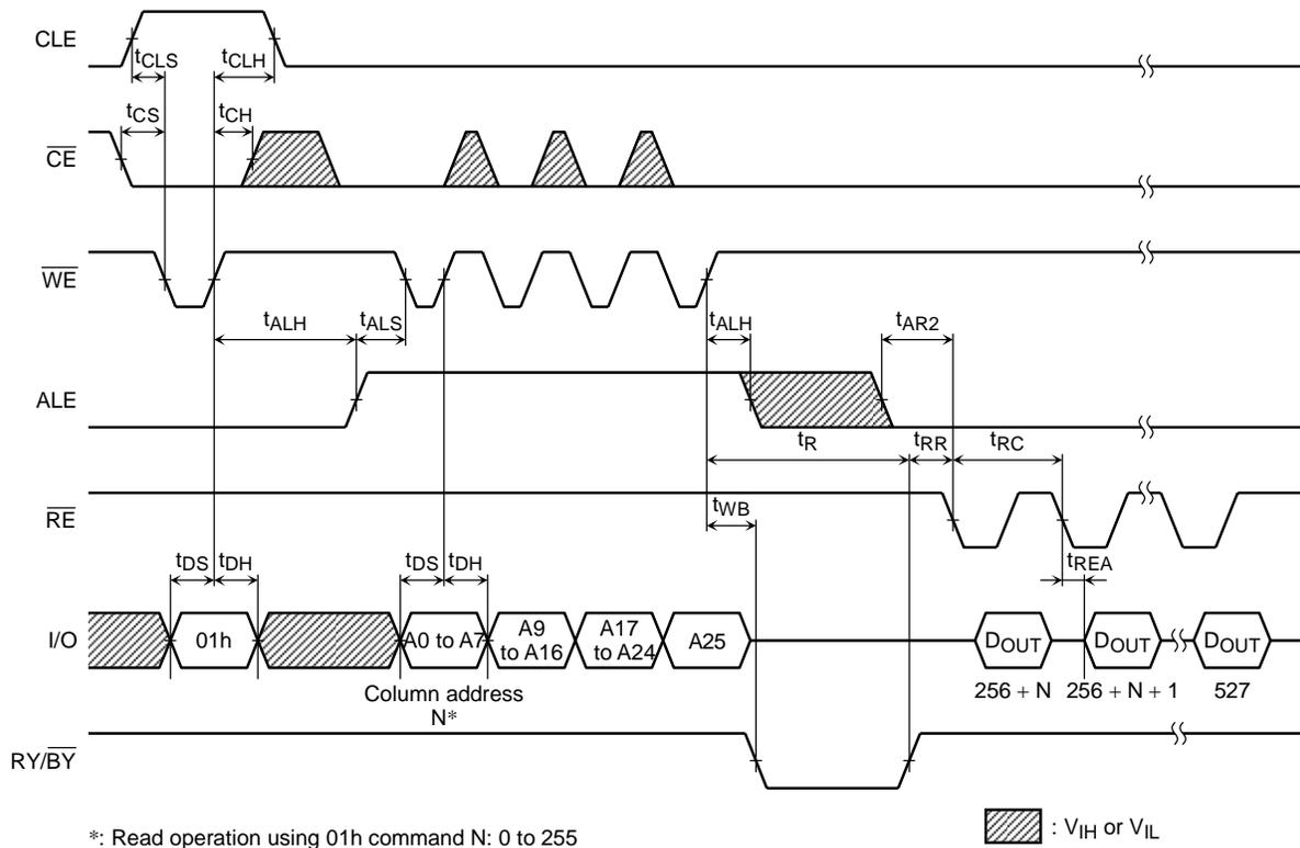
Read Cycle (3) Timing Diagram
