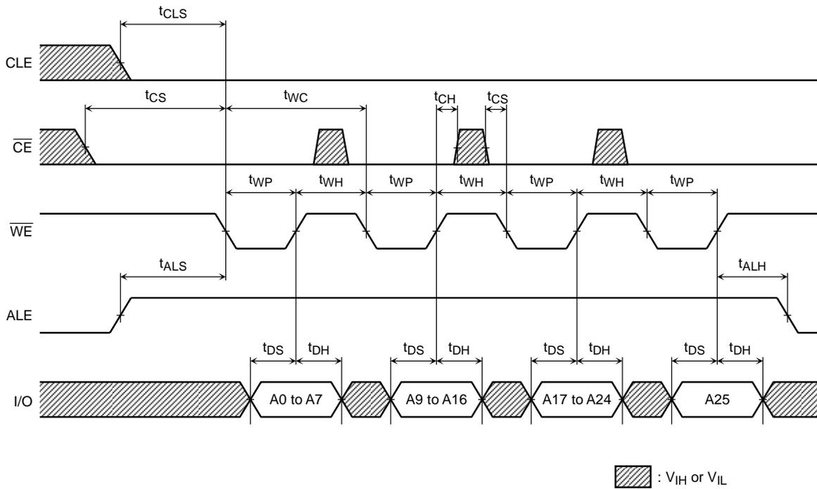
Data Input Cycle Timing Diagram
