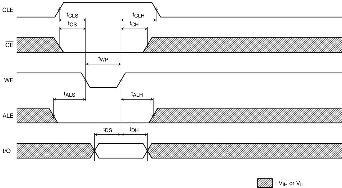
Address Input Cycle Timing Diagram
