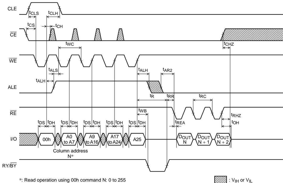
Read Cycle (2) Timing Diagram
