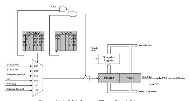
Figure 16.2. PCA Counter/Timer Block Diagram
