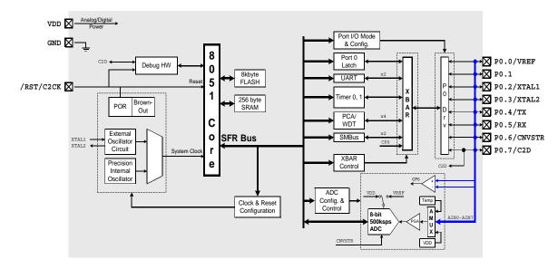
Figure 1.1. C8051F300/2 Block Diagram
