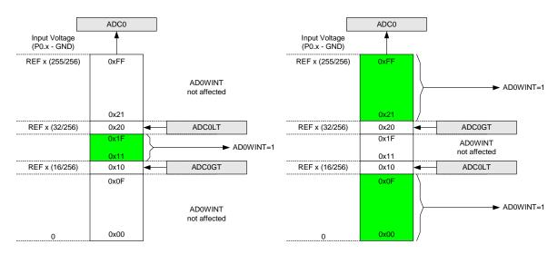
Figure 5.6. ADC Window Compare Examples, Single-Ended Mode
