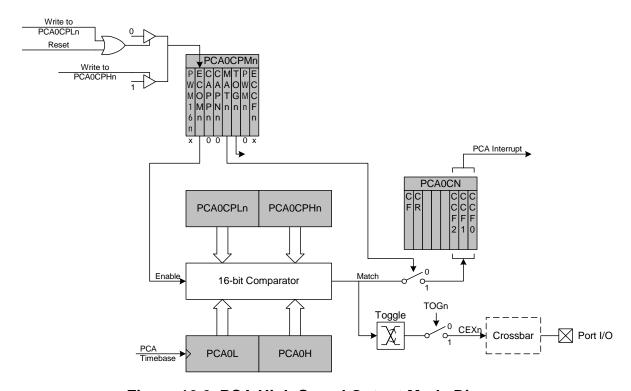
Figure 16.6. PCA High Speed Output Mode Diagram
