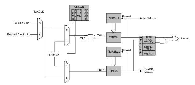
Figure 15.5. Timer 2 8-Bit Mode Block Diagram
