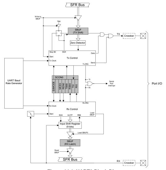
Figure 14.1. UARTO Block Diagram
