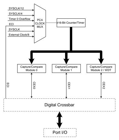
Figure 16.1. PCA Block Diagram
