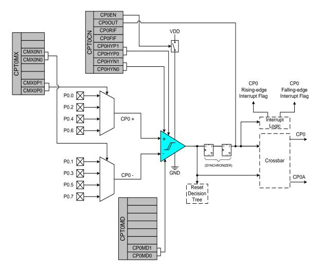
Figure 7.1. Comparator Functional Block Diagram
