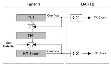
Figure 14.2. UARTO Baud Rate Logic
