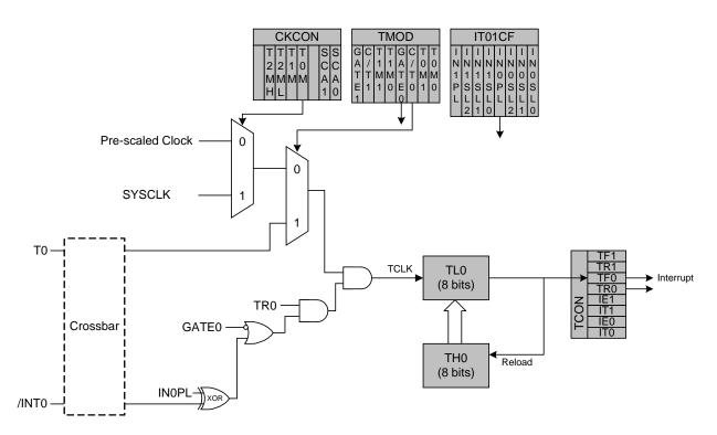
Figure 15.2. T0 Mode 2 Block Diagram
