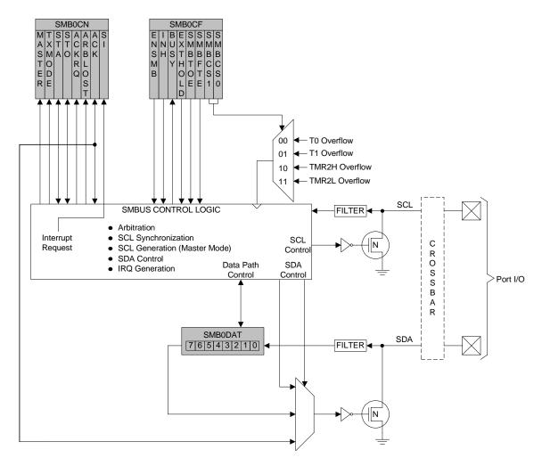
Figure 13.1. SMBus Block Diagram
