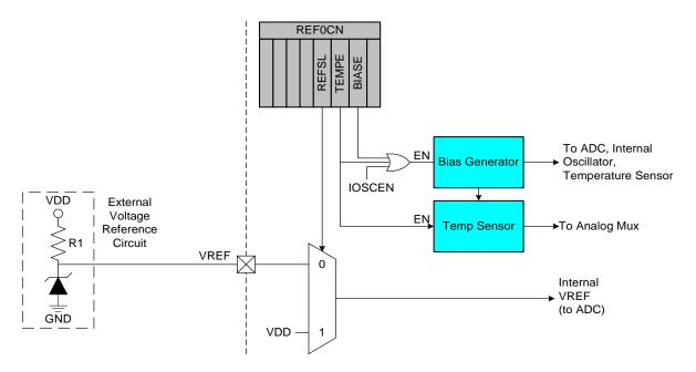
Figure 6.1. Voltage Reference Functional Block Diagram
