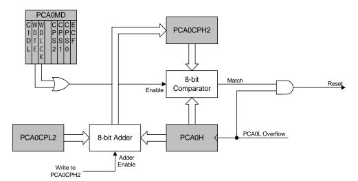
Figure 16.10. PCA Module 2 with Watchdog Timer Enabled
