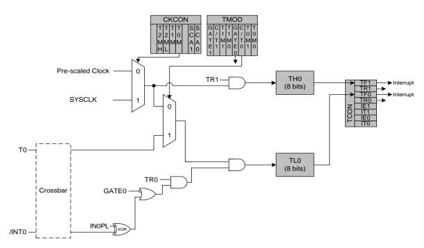
Figure 15.3. T0 Mode 3 Block Diagram
