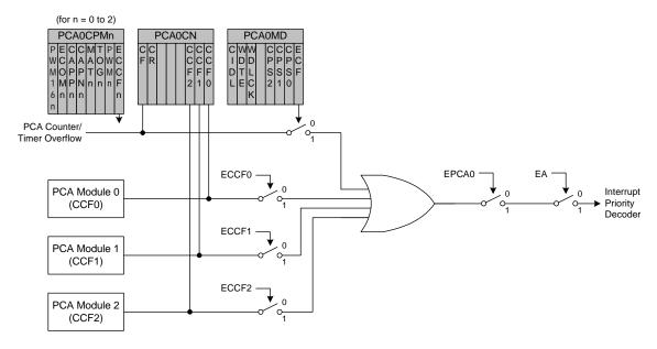
Figure 16.3. PCA Interrupt Block Diagram
