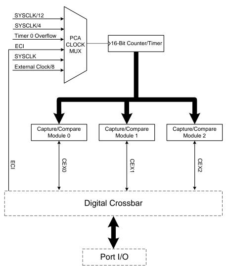
Figure 1.9. PCA Block Diagram
