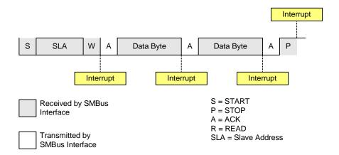
Figure 13.7. Typical Slave Receiver Sequence
