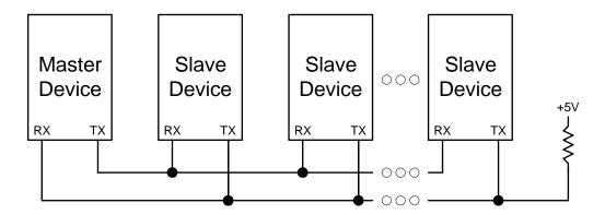
Figure 14.6. UART Multi-Processor Mode Interconnect Diagram
