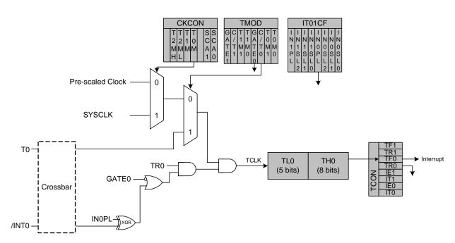
Figure 15.1. T0 Mode 0 Block Diagram
