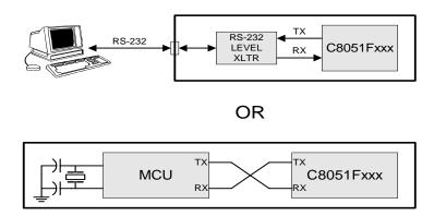
Figure 14.3. UART Interconnect Diagram
