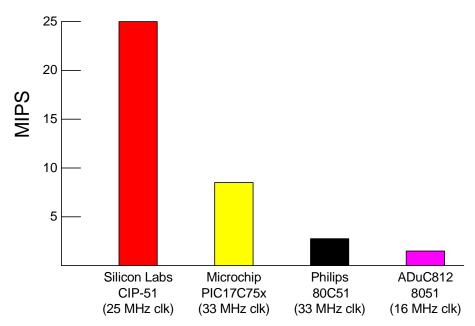
Figure 1.3. Comparison of Peak MCU Execution Speeds
