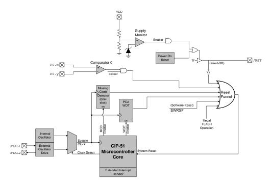
Figure 1.4. On-Chip Clock and Reset
