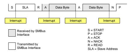
Figure 13.6. Typical Master Receiver Sequence
