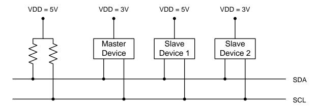
Figure 13.2. Typical SMBus Configuration
