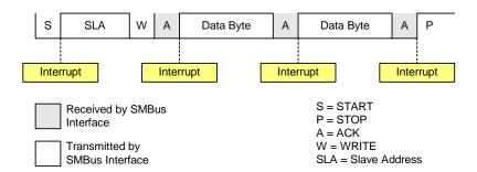
Figure 13.5. Typical Master Transmitter Sequence
