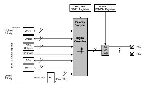
Figure 12.1. Port I/O Functional Block Diagram
