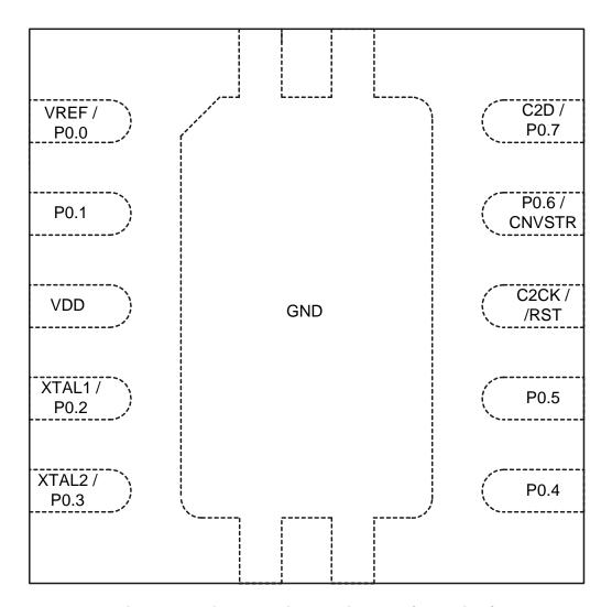
Figure 4.1. QFN-11 Pinout Diagram (Top View)
