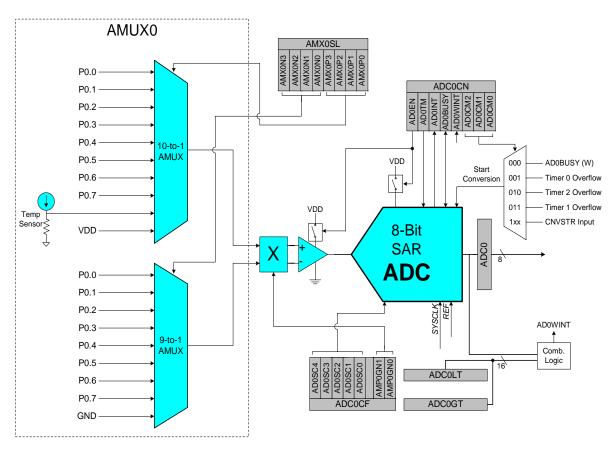
Figure 5.1. ADC0 Functional Block Diagram
