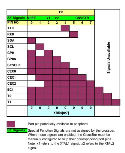
Figure 12.3. Crossbar Priority Decoder with XBR0 = 0x00
