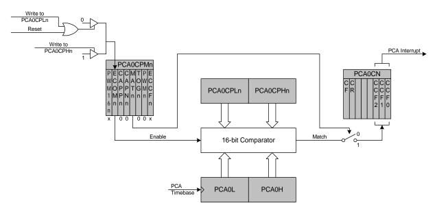
Figure 16.5. PCA Software Timer Mode Diagram
