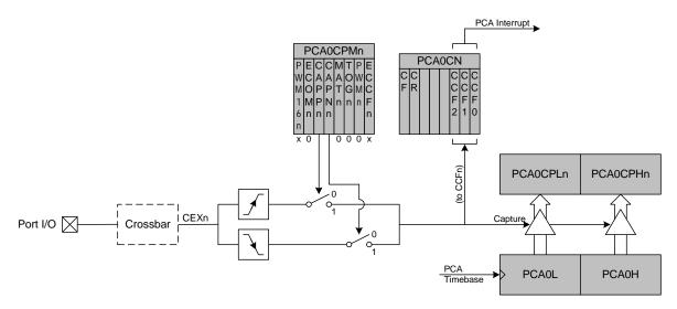
Figure 16.4. PCA Capture Mode Diagram
