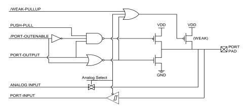
Figure 12.2. Port I/O Cell Block Diagram
