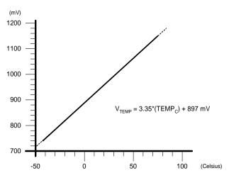
Figure 5.2. Typical Temperature Sensor Transfer Function
