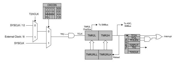
Figure 15.4. Timer 2 16-Bit Mode Block Diagram
