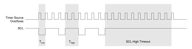
Figure 13.4. Typical SMBus SCL Generation
