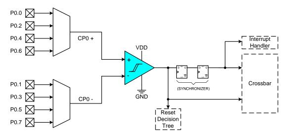
Figure 1.11. Comparator Block Diagram
