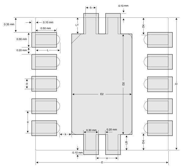
Figure 4.4. Typical QFN-11 Landing Diagram
