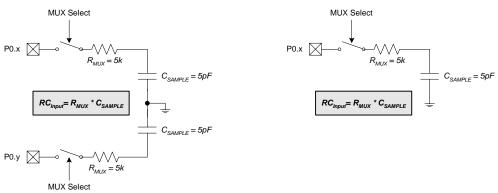
Note: When the PGA gain is set to 0.5,  $C_{SAMPLE} = 3pF$
