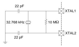
Figure 11.2. 32.768 kHz External Crystal Example
