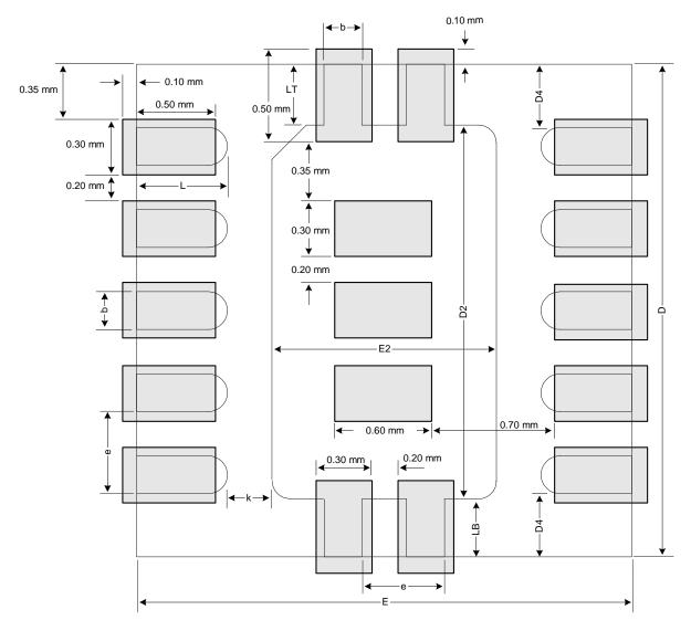
Figure 4.3. Typical QFN-11 Solder Paste Mask
