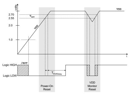
Figure 9.2. Power-On and V<sub>DD</sub> Monitor Reset Timing
