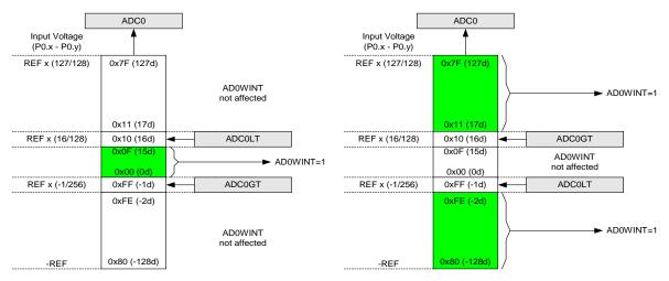
Figure 5.7. ADC Window Compare Examples, Differential Mode
