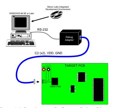
Figure 1.6. Development/In-System Debug Diagram
