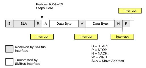
Figure 13.8. Typical Slave Transmitter Sequence
