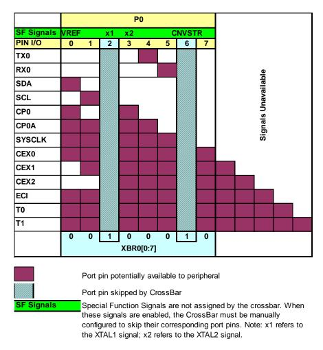
Figure 12.4. Crossbar Priority Decoder with XBR0 = 0x44
