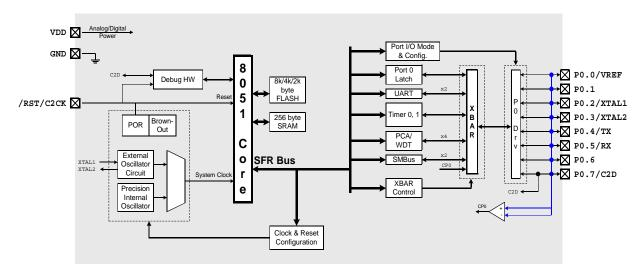
Figure 1.2. C8051F301/3/4/5 Block Diagram
