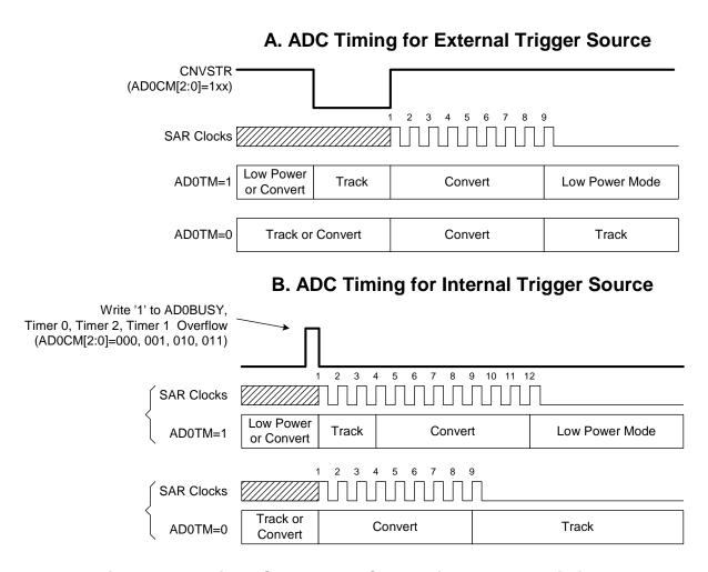
Figure 5.4. 8-Bit ADC Track and Conversion Example Timing
