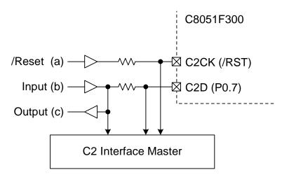
Figure 17.1. Typical C2 Pin Sharing
