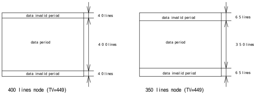
7-4. Input Data Signals and Display Position on the screen
