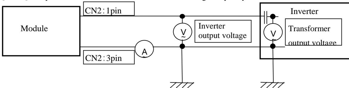
【Note2】 Referential data per one CCFT by calculation. ( $I_L \times V_L$ )
