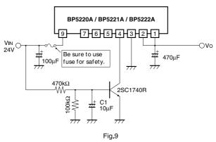
C1 is a slow-start capacitor for mitigating the over rush current that flows into the modules when the switch is turned on.
