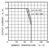
Fig.13 Derating curve
