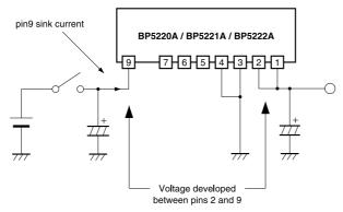
Fig.19 ASO measurement circuit
