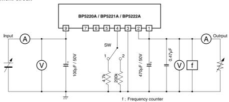
$100\mu\text{F/50V},\,470\mu\text{F/50V}$  ; PL series  $\diagup$  NICHIKON(Low-impedance type)
