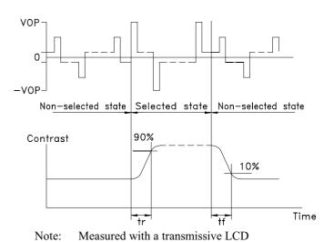
$V_{OPR}$  : Operating voltgae  $f_{FRM}$  : Frame frequency  $t_r$  : Response time (rise)  $t_f$  : Response time (fall)
