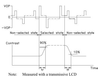
$V_{OPR}$  : Operating voltage  $f_{FRM}$  : Frame frequency  $Tr_{operation}$  : Response time (rise)  $tf_{operation}$  : Response time (fall)
