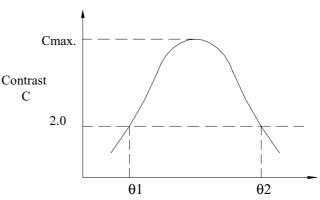
viewing angle  $\theta$  ( $\varnothing$  fixed) Note: Optimum viewing angle with the naked eye and viewing angle  $\theta$  at Cmax. Above are not always the same
