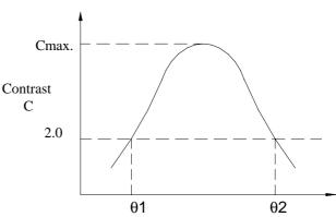
viewing angle  $\theta$  ( $\emptyset$  fixed) Note: Optimum viewing angle with the naked eye and viewing angle  $\theta$  at Cmax. Above are not always the same
