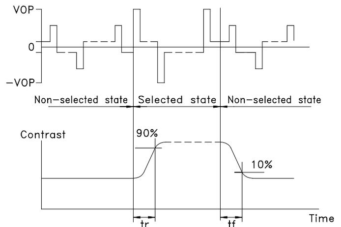
Note: Measured with a transmissive LCD panel which is displayed  $1 \text{ cm}^2$
