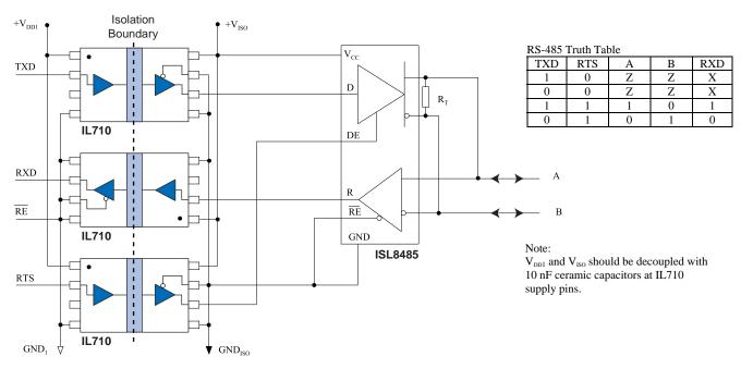
NVE offers a unique line of PROFIBUS/RS-485 transceivers, but IL710 isolators can also be used as part of multi-chip designs using non-isolated PROFIBUS transceivers.
