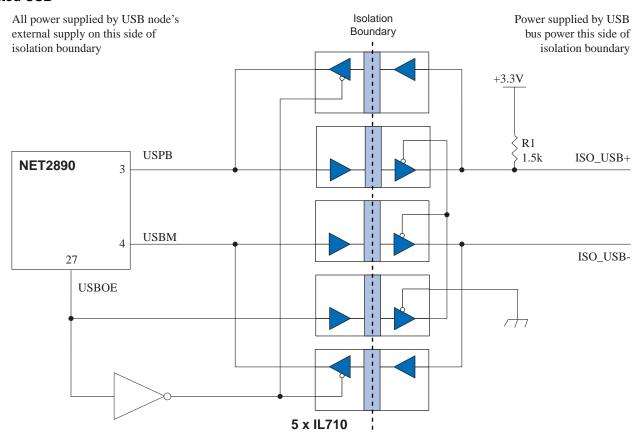
In this circuit, power is supplied by USB bus power on one side of the isolation barrier, and the USB node's external supply on the other side of the barrier. IL700 Isolators are specified with just 3 ns worst-case pulse width distortion.
