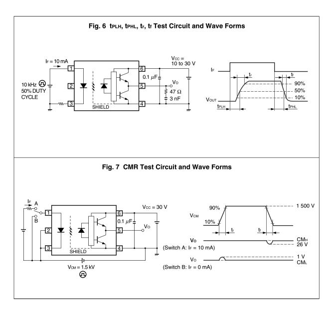
**Remarks 1.** Common Mode Transient Immunity at High Level Output is the maximum value of dVCM/dt at which the output remains High Level (e.g. Vo > 26 V).
