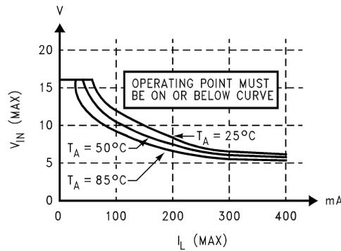
FIGURE 6. Safe Operation Boundary Curves for Figure 5
