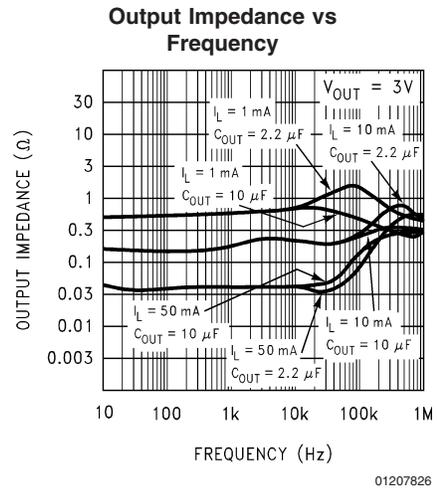
**Typical Performance Characteristics** Unless otherwise specified:  $T_A = 25^\circ\text{C}$ ,  $V_{IN} = V_{O(NOM)} + 1\text{V}$ ,  $C_{OUT} = 2.2 \mu\text{F}$ , all voltage options, ON/OFF pin tied to  $V_{IN}$ . (Continued)
