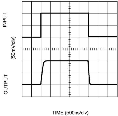
**Inverting Large Signal Pulse Response,  $V_S = 2.7V$**
