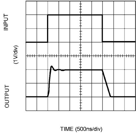
Non-Inverting Small Signal Pulse Response,  $V_S = 2.7V$
