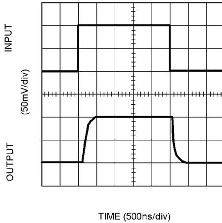
Non-Inverting Small Signal Pulse Response,  $V_S = 5V$
