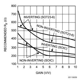
FIGURE 3. Recommended R<sub>F</sub> vs. Gain
