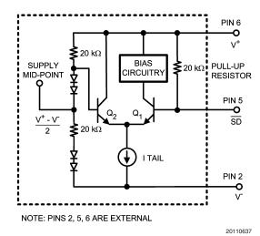
FIGURE 6. SD Pin Simplified Schematic (SOT23 Pinout Shown)
