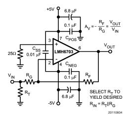
FIGURE 2. Recommended Inverting Gain Circuit (SOIC Pinout Shown)
