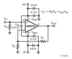
FIGURE 1. Recommended Non-Inverting Gain Circuit (SOIC Pinout Shown)
