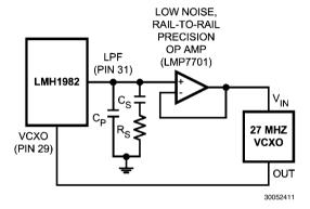
FIGURE 2. Optional Buffer to Isolate VCXO Input Impedance from the Loop Filter
