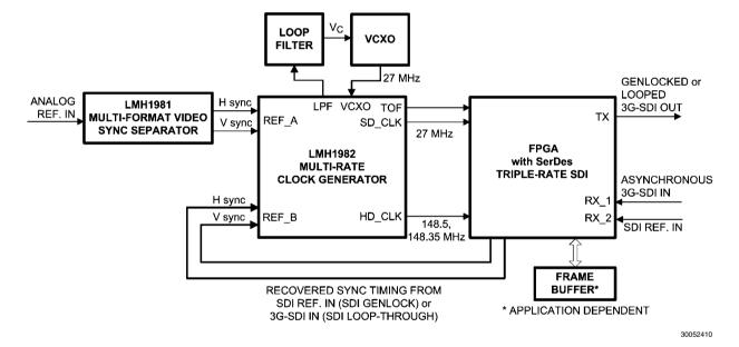
FIGURE 12. Combined Genlock or Loop-through for Triple-rate SDI Video
