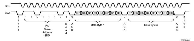
FIGURE 8. LMH1982 Read Sequence - Data Read Transfer
