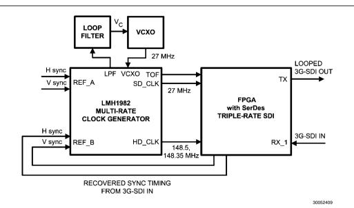
FIGURE 11. Triple-rate SDI Loop-through
