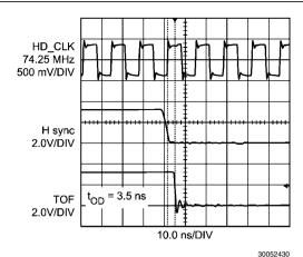
FIGURE 4. 1080i50 TOF Output Delay Time Relative to 74.25 MHz
