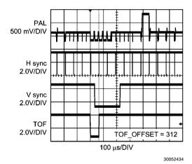
FIGURE 5. PAL Reference and Output TOF Pulse (TOF\_OFFSET = 312)
