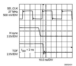
FIGURE 3. 525i TOF Output Delay Time Relative to 27 MHz
