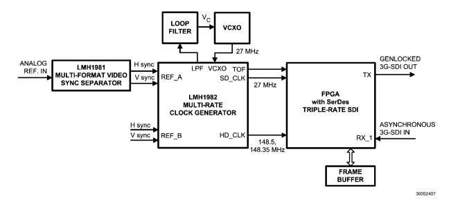
FIGURE 9. Analog Reference Genlock for Triple-rate SDI Video
