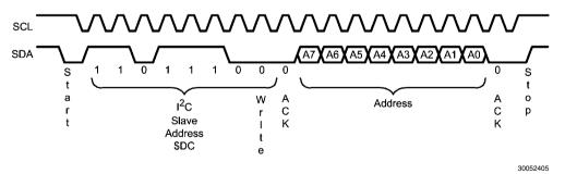
FIGURE 7. LMH1982 Read Sequence - Address Access Transfer
