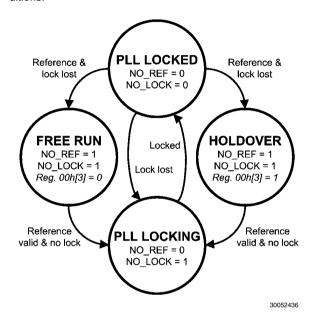
FIGURE 1. Genlock Mode State Diagram
