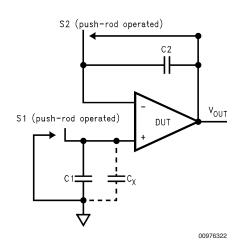
FIGURE 11. Simple Input Bias Current Test Circuit
