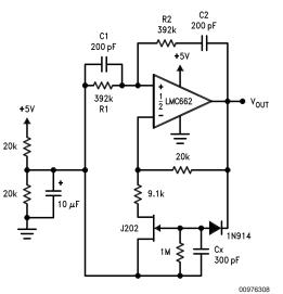
Oscillator frequency is determined by R1, R2, C1, and C2:
