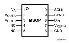
DAC102S085 10-Bit Micro Power DUAL Digital-to-Analog Converter with Rail-to-Rail Output
