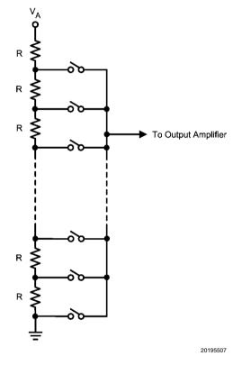
FIGURE 3. DAC Resistor String
