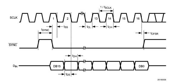
FIGURE 2. Serial Timing Diagram
