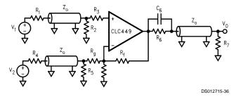
FIGURE 6. Transmission Line Matching
