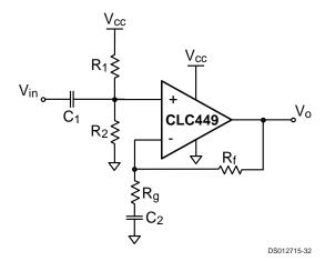
FIGURE 4. Single Supply Circuit
