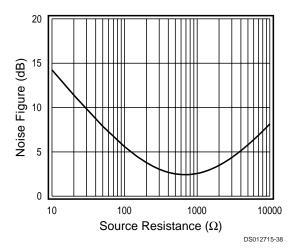
FIGURE 7. Noise Figure Plot
