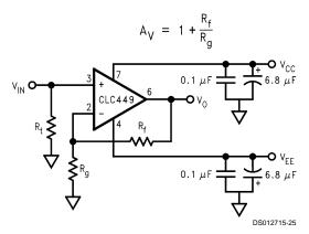
FIGURE 1. Non-Inverting Gain
