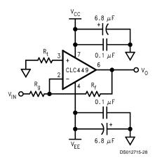
FIGURE 2. Inverting Gain
