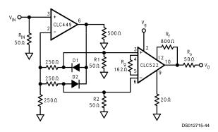
FIGURE 10. Full-Wave Rectifier
