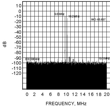
**Crosstalk Response  $f_{IN} = 9.95\text{ MHz}$ ,  $f_{CROSSTALK} = 15\text{ MHz}$ ,  $f_{CLK} = 40\text{ MHz}$**
