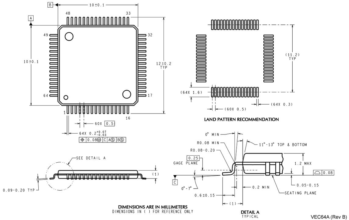
**64-Lead TQFP Package**
