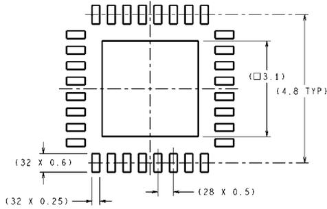
**DIMENSIONS ARE IN MILLIMETERS**
