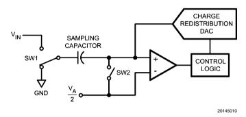
FIGURE 4. ADC121S101 in Hold Mode
