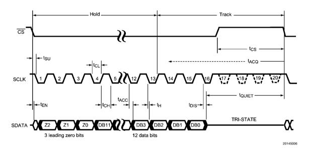
FIGURE 2. ADC121S101 Serial Timing Diagram
