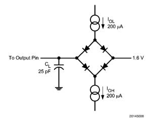
FIGURE 1. Timing Test Circuit
