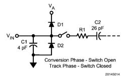
FIGURE 7. Equivalent Input Circuit
