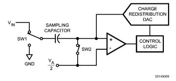
FIGURE 3. ADC121S101 in Track Mode
