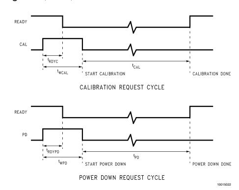
FIGURE 4. Reset and Calibration Timing
