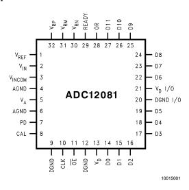
ADC12081 12-Bit, 5 MHz Self-Calibrating, Pipelined A/D Converter with Internal Sample & Hold
