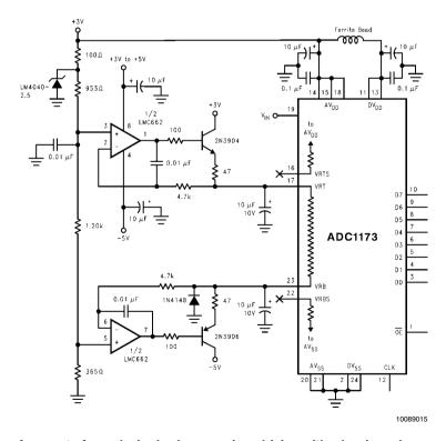
FIGURE 5. Driving the reference to force desired values requires driving with a low impedance source, provided by the transistors. Note that pins 16 and 22 are not connected.
