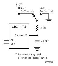
FIGURE 2.  $t_{EN}$ ,  $t_{DIS}$  Test Circuit
