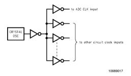
FIGURE 6. Isolating the ADC clock from Digital Circuitry.
