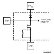
Note 8: To guarantee accuracy, it is required that  $AV_{DD}$  and  $DV_{DD}$  be well bypassed. Each supply pin must be decoupled with separate bypass capacitors.
