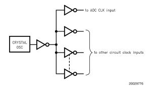
FIGURE 9. Isolating the ADC Clock from Digital Circuitry
