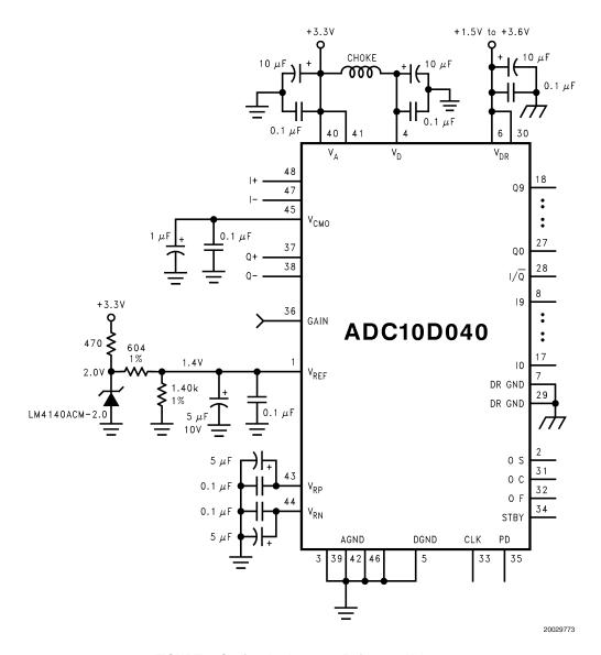
FIGURE 6. Setting An Accurate Reference Voltage
