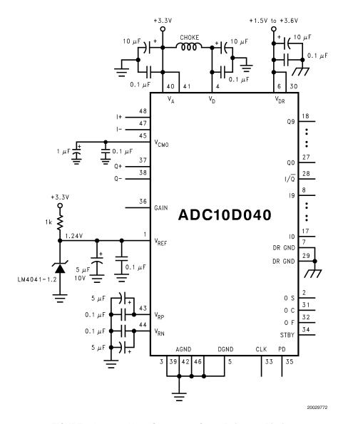
FIGURE 5. Improved Low Component Count Reference Biasing
