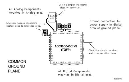
FIGURE 8. An Acceptable Layout Pattern
