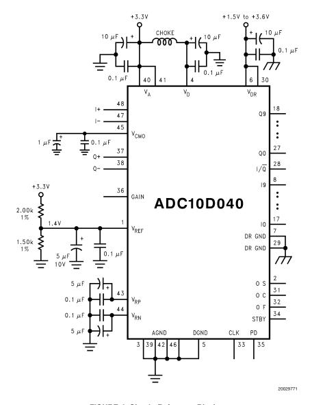
FIGURE 4. Simple Reference Biasing
