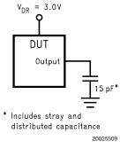
FIGURE 1. AC Test Circuit
