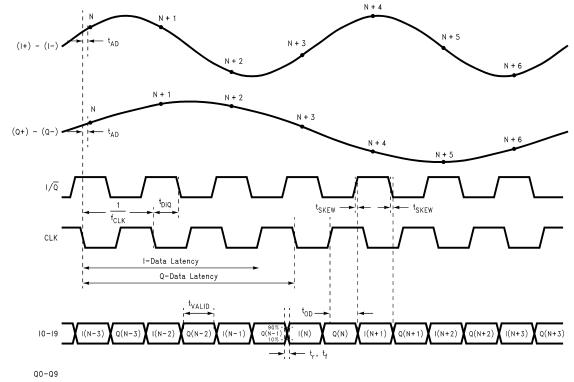
ADC10D020 Timing Diagram for Multiplexed Mode
