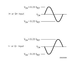
FIGURE 2. The ADC10D020 is designed for use with differential signals of 1.0  $V_{P-P}$  with a common mode voltage of 1.5V. The signal swing should not cause any pin to experience a swing more than 300 mV beyond the supply rails.
