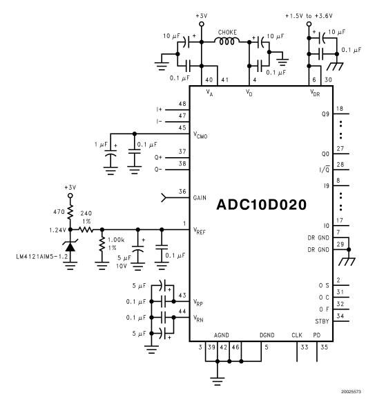
FIGURE 6. Setting An Accurate Reference Voltage
