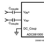
FIGURE 4. Differential Input Drive
